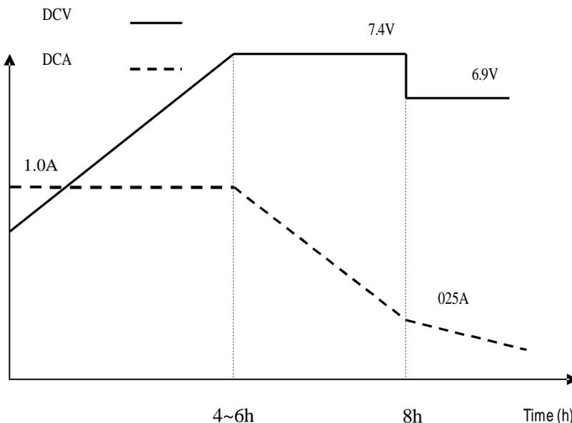
**Note:** this chart is for 6V5AH battery, 1 pcs use, for other 12V battery, the charging time should be adjusted accordingly.
